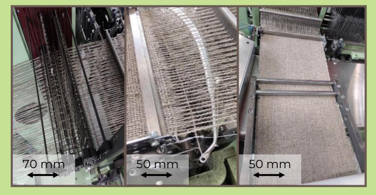
Samples were produced using a narrowband needle loom using four harnesses and a plain weave structure.
