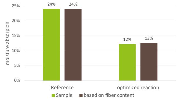
The comparison of untreated hemp fibers with treated and cavity filled natural fibers shows a reduction of 50% moisture absorpion.
